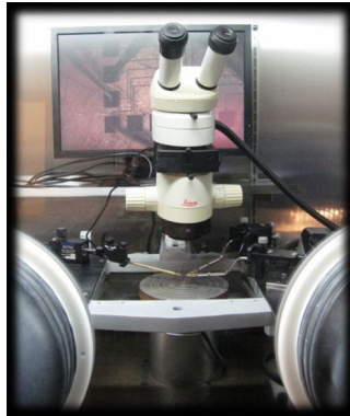
Point station in glove box
