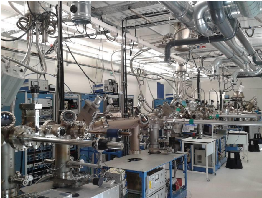
UHV cluster: MBE (III-V + oxides) + sputtering + XPS (+ ALD)
